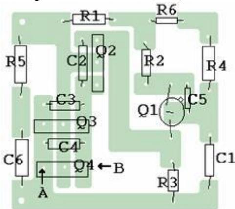
If you only intend to use a single lamp, Q2 C2 Q3 C3 may be omitted. Connect a jumper between A and B as shown on the component layout diagram.
