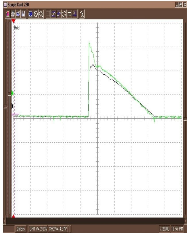
Power through  $2\Omega$  between APS and lamp measured with Scope Card 220. V1 and V2 are sampled from waveforms. Sample voltages summed are  $V1 = 737.47$   $V2 = 779.69$ . Dividing by No. of samples (20) is  $V1 = 38.98$   $V2 = 36.87$ .
