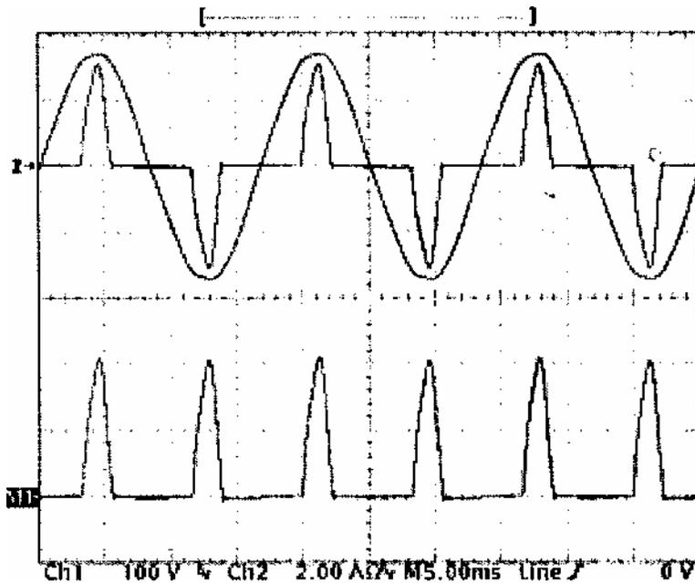
The upper waveforms are the voltage and current scaled at 100 V per division and 2 A per division. The scope multiplies the voltage and current to create the instantaneous power waveform (lower).
