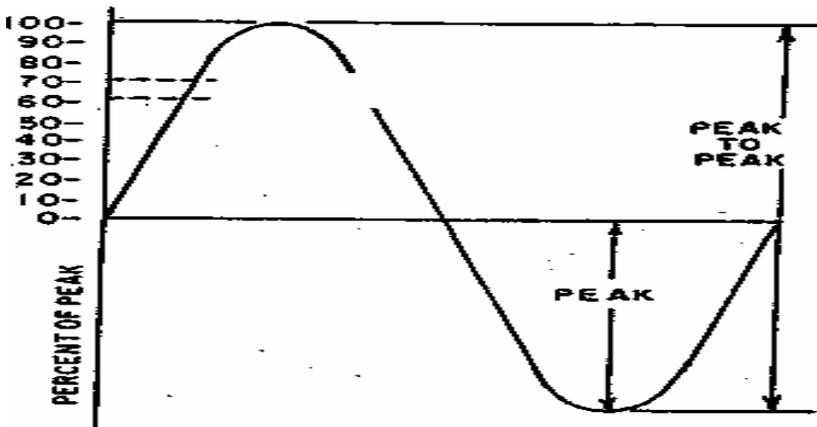
compute the average value of one alternation. This could be accomplished by adding together, a series of instantaneous values of the wave between  $0^\circ$  and  $180^\circ$ , and then dividing the sum by the number of instantaneous values used. Such a computation would show one alternation of a sine wave to have an average value equal to 0.637 of the peak value. In terms of an equation:  $E_{av} = 0.637 E_m$ .
