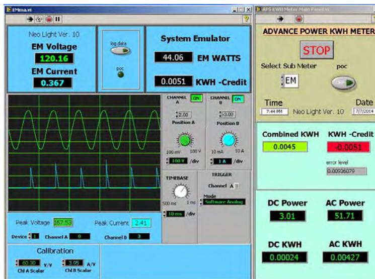
Measures offset encountered in operations with industry KWH meters. The error level is computed and processed to deliver a credit reflecting true power rather than RMS power. A negative credit in KWH is displayed on the first front panel and is applicable during operations to assure the consumer is billed correctly.
